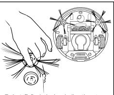
**To Install:** Push the brush directly onto the holder.
