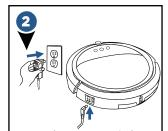
Leave the power switch on and charge the battery directly from power cord for 4-5 hours prior to the first operation.
