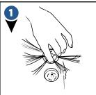
Install the edge cleaning brushes and the battery according to the assembly instructions.
