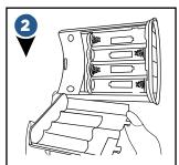
Insert batteries with the +/- terminals facing the directions indicated and replace the battery cover. (AA batteries not included)
