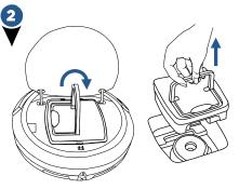
Pull up the dust bin handle and take out the dust bin from the robot.
