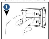
To remove the battery cover, hold the invisible wall and press firmly while sliding downward to remove the battery cover.
