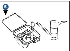
Rinse the dust bin with tap water. It is not necessary to wash every time.
