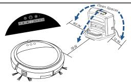
To test the auto-charge feature of the dock, turn the power switch ON and select "00" with the center button (see page 9 for control panel details). The vacuum should back into the dock for recharging if the appropriate spacing was provided for the docking station.
