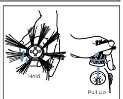
**To Remove:** Hold the brush bristle and pull upward to remove the brush.
